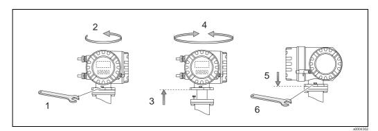
*Fig. 24: Turning the transmitter housing (aluminum field housing)*
