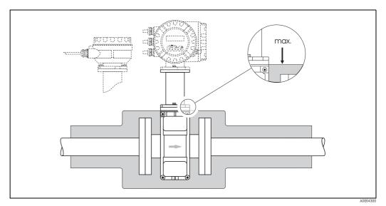
Fig. 21: Promag P (high-temperature version): Insulating the pipe
