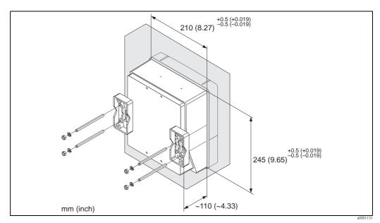
Fig. 28: Panel installation (wall-mount housing)
