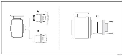
Abb. 22: Promag H process connections (DN 2...25 / DN 40...100, 1/12"...1" / DN 11/2"...4")
