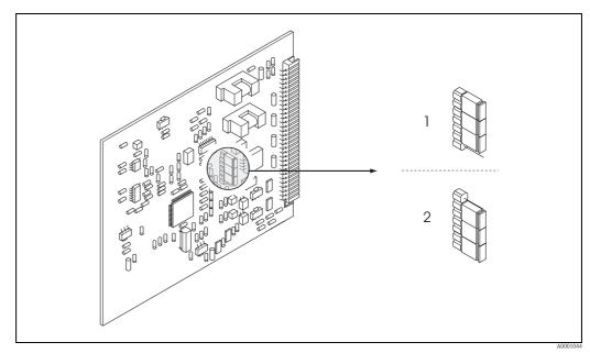
*Fig. 51:* Configuring current outputs using jumpers (I/O board)
