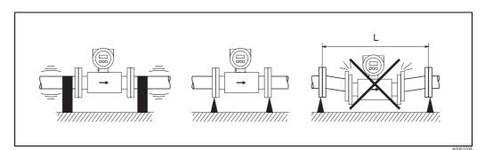
Fig. 13: Measures to prevent vibration of the device (L > 10 m (32.8 ft))
