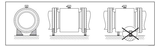
Fig. 14: Correct support for large nominal diameters ( $DN \ge 350$ )
