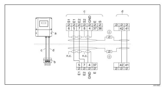
*Fig. 30:* Connecting the remote version of Promag D
