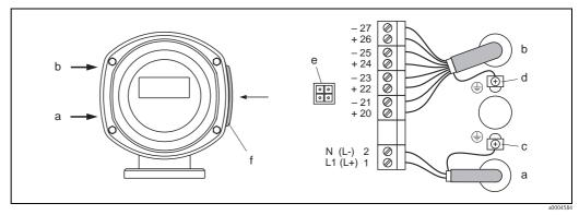
*Fig. 35:* Connecting the transmitter (stainless steel field housing); cable cross-section: max. 2.5 mm<sup>2</sup>
