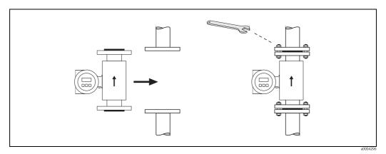
Fig. 18: Installing the Promag L sensor
