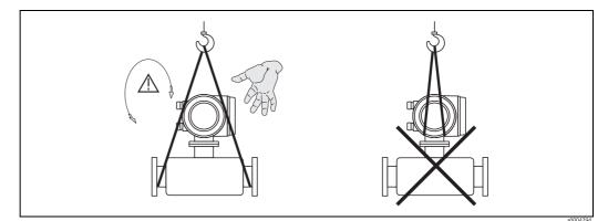
*Fig. 4:* Transporting sensors with  $DN \le 300 \ (\le 12")$
