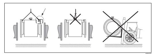
*Fig. 5:* Transporting sensors with DN > 300 (> 12")
