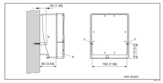
Fig. 27: Mounted directly on the wall
