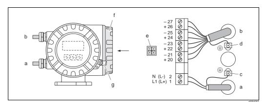
Fig. 34: Connecting the transmitter (aluminum field housing). Cable cross-section: max. 2.5 mm<sup>2</sup>
