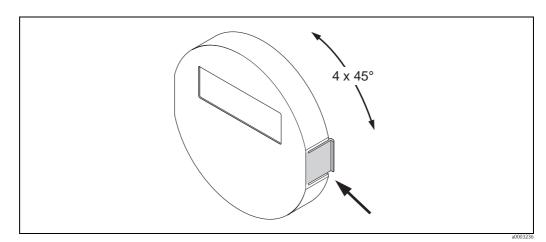
Fig. 26: Turning the local display (field housing)
