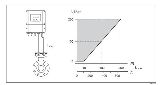
Fig. 16: Permissible cable length for the remote version
