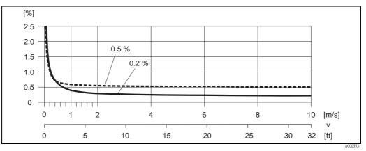
Max. measured error in % of reading Fig. 57:
