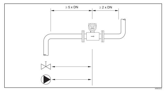
Fig. 12: Inlet and outlet runs
