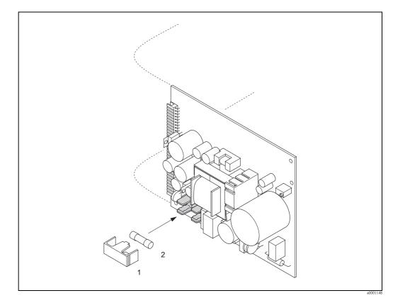
Fig. 55: Replacing the device fuse on the power supply board
