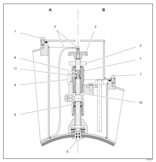
Fig. 56: Apparatus for replacing exchangeable measuring electrodes
