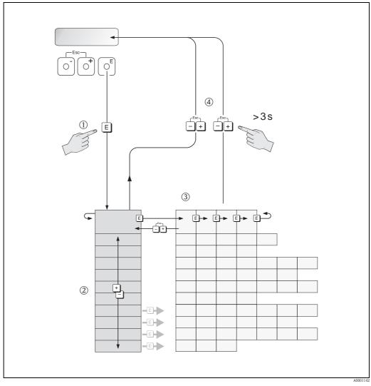
Fig. 48: Selecting functions and configuring parameters (function matrix)
