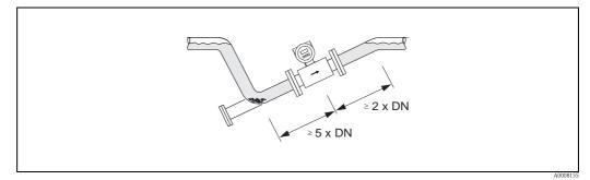
*Fig. 8: Installation in a partially filled pipe*
