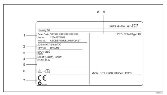
Fig. 1: Nameplate specifications for the "Promag 50" transmitter (example)
