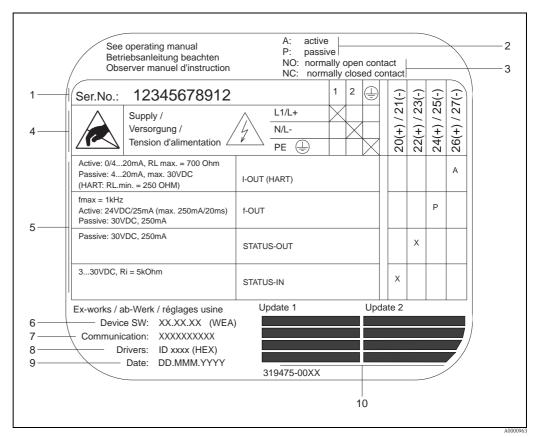
*Fig. 3:* Nameplate specifications for transmitter (example)
