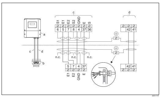
Fig. 32: Connecting the remote version of Promag H
