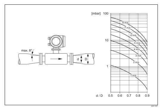
*Fig. 15: Pressure loss due to adapters*
