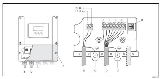
Fig. 36: Connecting the transmitter (wall-mount housing); cable cross-section: max. 2.5 mm<sup>2</sup>
