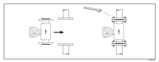
Fig. 20: Installing the Promag P sensor
