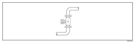
Fig. 10: Vertical orientation
