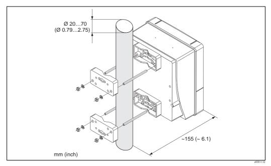
Fig. 29: Pipe mounting (wall-mount housing)
