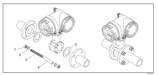
Fig. 17: Mounting the sensor
