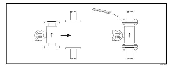
Fig. 19: Installing the Promag W sensor
