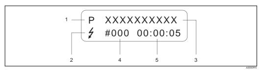
Fig. 49: Error messages on the display (example)
