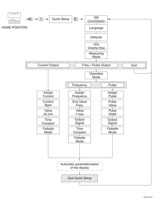
Fig. 50: "OUICK SETUP COMMISSIONING" menu for the rapid configuration of important device functions
